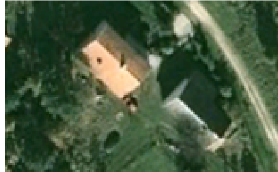
This photo is properly projected on elevation model, yet on a single building scale, a small tilt is noticeable. This is an Orthophoto, but not a True Orthophoto (not all vertical features are reprojected).
